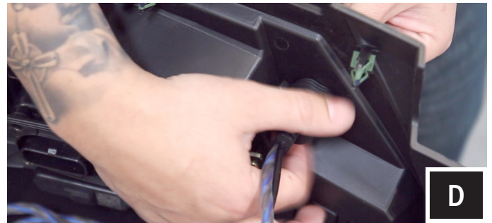
D. Feed the plastic nut back through the wires and cables and screw back onto the port. Hand tighten only. Replace fuse and close fuse holder.
