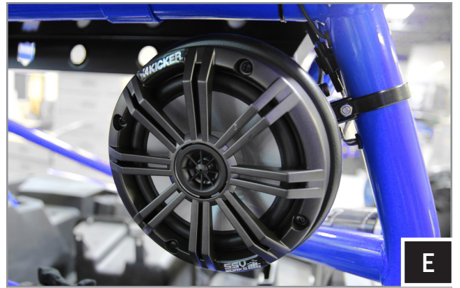
E. Route the speaker wire away from any moving parts and any sharp metal, then connect to the amplifier
