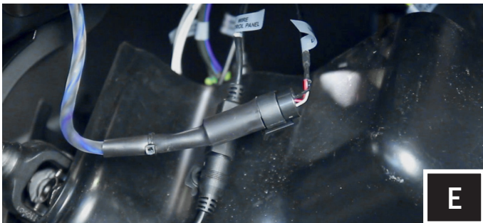
E. Connect the AUX-in connector to the MRB3 brain.
