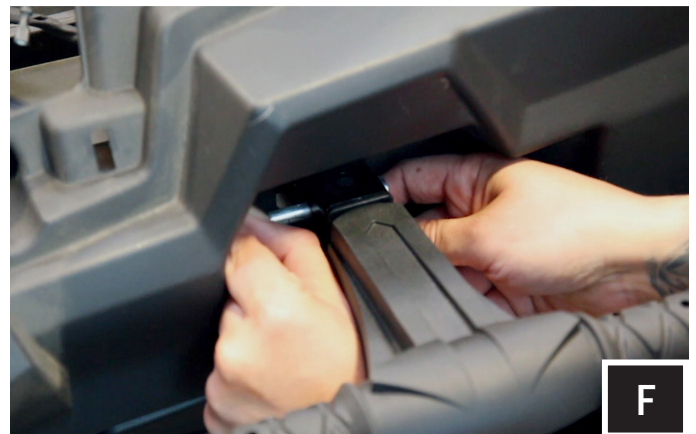
F. Un-pin and pull to remove the passenger side safety handle.
