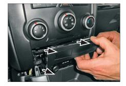
Unclip panel holding the cigarette lighter and remove it (pull out plugs carefully)
