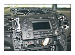
9. Remove screws of OEM radio
