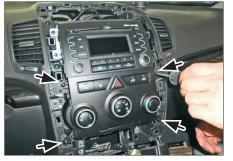
control unit and remove it (pull out plugs carefully)
