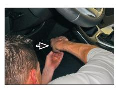
Remove plastic rivets at left and right side. remove panels
