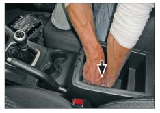
Remove plastic cover remove 3 screws
