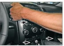
Remove screws of air condition
