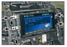
10. Fix mounting brackets to Double DIN Navigation
