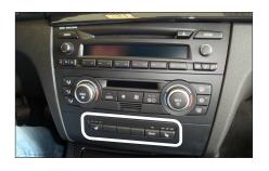
1. BMW 1 (E87) 03/2007 (facelift) with switch bar under the climate control unit
