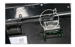
5 Unclip and remove switch panel below air condition control unit
