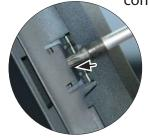
7. Remove screws below OEM head unit (see arrows)
