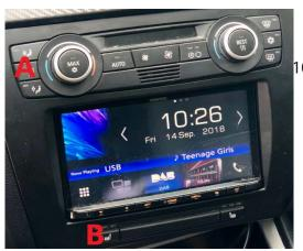
10. Attach air condition control unit(a) and switch bar (b) toreplacement facia plate
