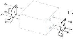
11. Attach mounting brackets to double DIN navigation
