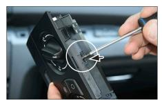
5. Unclip and remove air condition control unit
