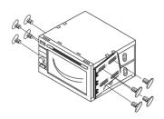
11. Mount the DDIN radio to the supplied DDIN brackets using ISO screws.
