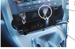
3. Remove the two screws below the OEM head unit
