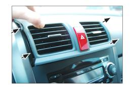
4. Remove the air vent unit
