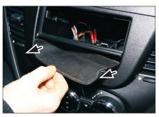
Remove anti-slip mat (fixed with double-sided tape)
