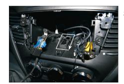
Remove OEM panel Cut away plastic in order to clear space for 2-DIN head unit
