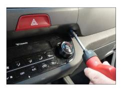
Remove screws of OEM head unit (left and right)
