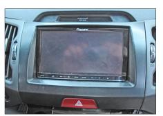
11. Remove hazard light switch (1) from OEM head unit - attach it to double DIN facia plate
