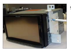
Attach metal mounting brackets to Double DIN Navigation
