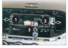
3. Remove screws of OEM head unit (1 + 2)
