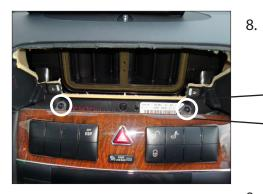
Remove the two Torx screws, located over the switch panel. Remove the switch panel.
