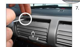
Unclip the air vent unit carefully on both sides with a screw driver.
