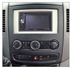
Push the Metal Frame into the facia plate
