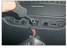
Remove screw under hazard light switch (see arrow)
