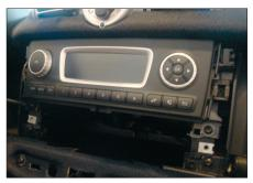
Remove screws of OEM head unit take out OEM head unit
