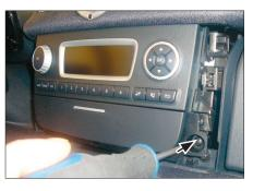
Remove screws of tray below OEM head unit (see arrows)
