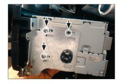
4. Fix mounting bracket left and mounting bracket right to double DIN head unit with 3 flat headed screws (see arrows) at each side
