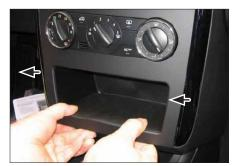
4. Unclip and remove lower panel
