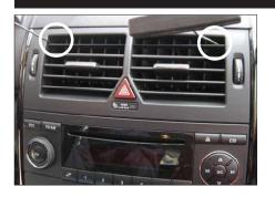
1. Insert pulling hooks into air vent catches. Pull out air vents
