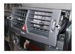
3. Remove air vents completely
