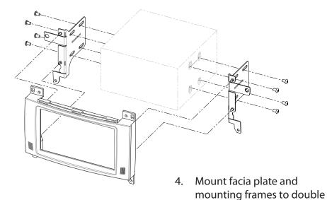
Connect all required circuit points and push double DIN head into dash board
