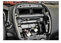
Dashboard with removed 3. OEM Radio/CD device
