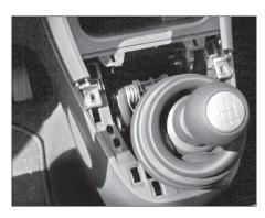
3. Remove the gear lever cap.
