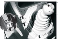
2. Remove the 2 screws left and right at the base of the silver trim frame.
