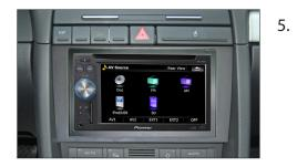
. Connect alle required circuit points and push the double DIN head unit until it snaps in.
