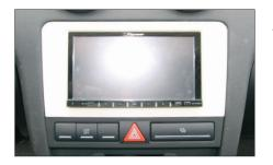
5. Connect alle required circuit points and push the double DIN head unit until it snaps in.
