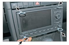
2. Use 4 radio release keys to dismount the OEM radio.
