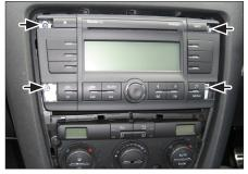
Remove 4 screws fixing the OEM head unit.
