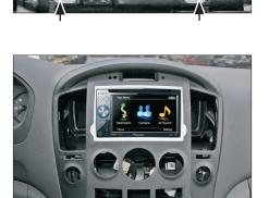
5. Place the 2-DIN Navigation with the facia plate at he dash board
