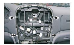
3. Unclip the front panel and remove it
