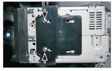
5. Put the mounting brackets on the Double-DIN head unit and fix it with the supplied screws.
