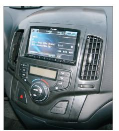
6. Place the Double-DIN head unit at the dashboard and fix it with the 4 original screws.
