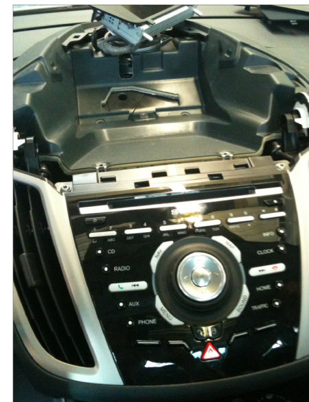
12. Remove screws on top of OEM head unit (left and right)
