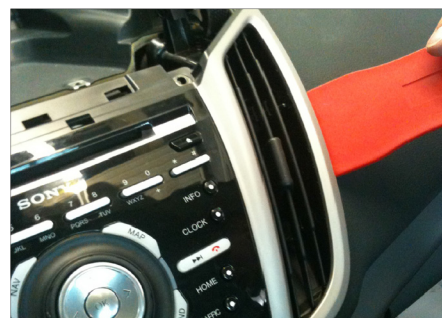
13. Unclip air vents Remove air vents
