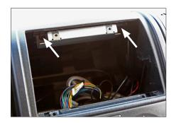
Assemble speed nuts on mounting plate Install mounting plate on top of dash board hole.
