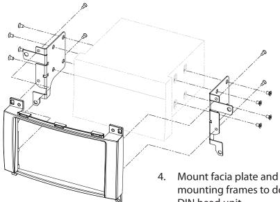
mounting frames to double DIN head unit
