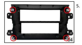
Apply the 4 clips removed previously to the new Halo frame.
