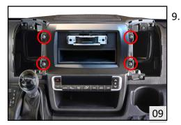
Make all connections. Fix the head unit with the OEM screws saved in the step n°3 as indicated in the picture.
