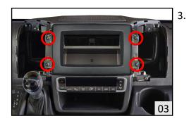
Remove and save the 4 screws circled in Red. Disengage the ISO connector from the OEM facia plate.
