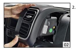
Disengage both air vents with a removal tool and remove both air vents.
