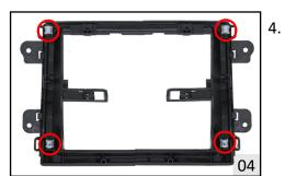
. Remove and save the 4 clips circled found to the back side of the OEM facia plate.
