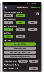
The basic settings (preferences) cover color selection for remote control and amp, converter filter characteristics, and buttons for adjusting the sensitivity of inputs and outputs
