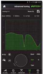
The 21 + 10 EQs at the inputs and outputs can be used as fully parametric EQs or shelving
