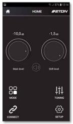
The Home screen provides level control for the Stealth and the subwoofer output. From here sub-menus can be accessed for source selection and settings
